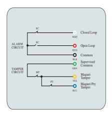
Dual alarm contacts both closed loop, with tamper circuit, closed loop. For built-in EOL resistor configurations and values not shown, contact Potter.
