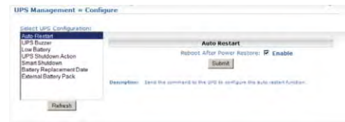
UPS/SNMP configuration screen (NV6)
