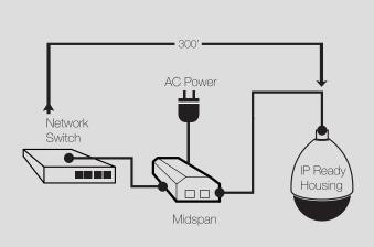
The distance from Network Switch to Camera Housing should be  $\leq$  300'
