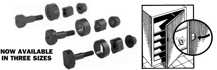
Major Manufacturing's punch and die set will punch a **DOUBLE "D"** hole in sheet metal cabinet drawers and doors. A must have tool for the locksmith working on vending machines, lockers, metal cabinets or any type of sheet metal door made with 18 guage (.048) or lighter steel. To use, simply drill a 1/2" hole centered where the cam lock is to be installed, slide the punch through the hole and tighten down the hex nut with a 11/16" wrench or socket set.
