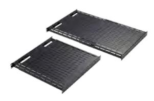
An easy-to-install tool-less vented 19-in. shelf. Mounts onto rack angles that have EIA-spaced square holes (.375 in.). Shelf slides open and provides a variable-sized, continuous surface for equipment. Back of shelf has oval cutouts for power and data cables. Accessory hole patterns at back of shelf fit small and large D-rings to help manage cable. Made of steel with a 150 lb. (68 kg) static load rating. Available with RAL 9005 black or RAL 7035 gray polyester powder coat finish.
