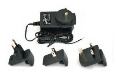
The ComNet™ PS12DC-1A-UNI has a removable pin head to allow it to use one of four different outlet configured pin heads to supply 12V DC power to ComNet stand-alone units. The PSU can also accept a standard figure 8 line cord input. Pin heads for the UK and Europe will be included as standard. The US and Australian heads are available upon request at no extra charge.
