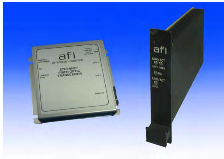
The American Fibertek 48 Series transmits and receives (2) copper 10/100/1000 BaseT Ethernet signals at the RJ45 ports and (1) optical 1000 Base-X over 1 or 2 multimode fibers. The system is comprised of two units forming a point-to-point communications link.
