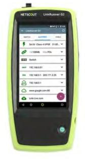
When customization of the AutoTest is needed, profiles can be defined to ensure a standardized test process is executed when variables about the link under test are needed. While these settings can be easily changed in use, profiles can be configured by a senior team member to ensure lessskilled technicians are executing an AutoTest that is specific to their network environment, which is particularly useful in organizations who manage distributed locations.
