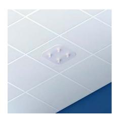
Cloud/canopy/suspended ceiling mounting kit for most vendors' APs and antennas. A cutout is made in the ceiling panel, the panel bridge is placed above the ceiling panel, and AP or antenna is attached to the white trim.
