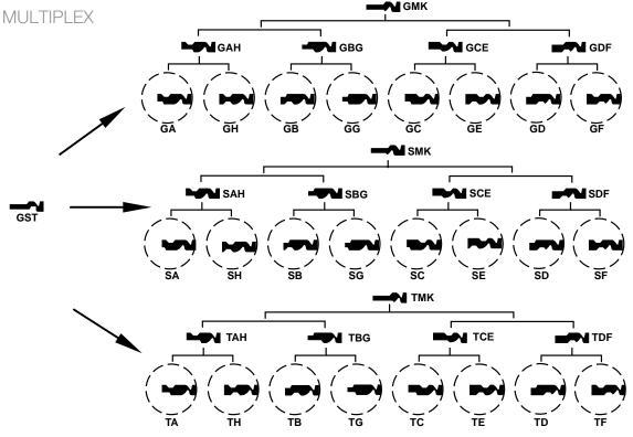
**Notes:** The section of the key is determined by viewing the key from the bow towards the tip. For security reasons, restricted and protected keyway profiles are not shown.
