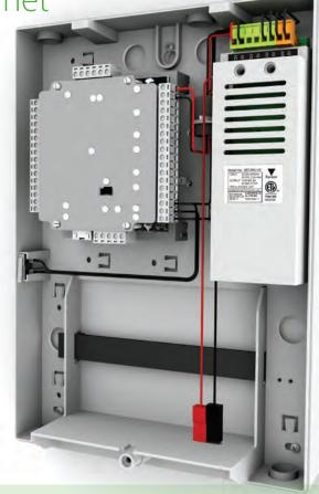
The 12/24V 2A AC/DC Power supply unit is available in either a plastic or metal cabinet. The cabinet can house both the 12/24V 2A AC/DC PSU and a Net2 ACU with the option to accomodate a 12V/7Ah back up battery if desired. A tamper switch is also installed which registers an alarm if the lid is opened when connected to an ACU. Please note that the Net2 nano ACU is not available for integration within the metal cabinet.
