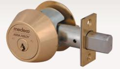
unique "captive thumbturn." The captive thumbturn converts the inside cylinder to a thumbturn for safe exit when the facility is occupied. A guick conversion when the facility is not occupied returns it to double cylinder mode and guards against unauthorized entry or exit. Maxum® deadbolts offer maximum protection with solid-brass construction, along with anti-drilling and anti-prying features.
