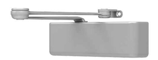
The 4510 SMOOTHEE® Series is a heavy duty, high security closer with special components to minimize tampering and vandalism. Forged steel double lever arms and heavy gauge metal security covers are designed for correctional, vandal prone, institutional and other high traffic applications. The closer has passed 10 million cycles in independent testing. A choice of finishes and cylinder functions meet correctional and vandal resistant requirements.
