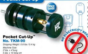
The Pocket Cut-Up™ is a compact, portable tubular key machine. It is factory preset to cut 7-pin standard, center sequence tubular keys by code. Offset left and offset right sequence (including dead pin cuts) can be cut with one simple adjustment. It also cuts Greenwald style tubular keys. The tubular key blank is held firmly in place by the swing-away key holding fixture, that locks the depth adjustment knob at
