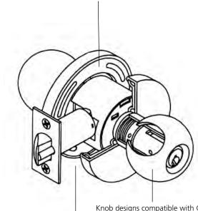
2-3/8" (60mm), 2-3/4" (70mm), 3-3/4" (95mm) – and 5" (127mm) backsets available Knob designs compatible with Corbin Russwin Pre-Assembled Unit Locks, Mortise Locksets, Exit Devices and other Cylindrical Locks
