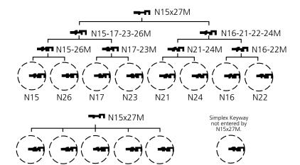
\*NOTE: Do not use these pairs in the same keying system with each other: N15 with N27; N17 with N19; N21 with N25
