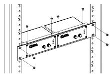
TSD-RRMK Optional Rear Rack Mounting Kit - For complete flexibility in mounting a TSD or TSD external power supplies the optional TSD-RRMK is available. The TSD-RRMK can support mounting of either two larger TSDs with external power supplies or up to 4 TSD models. **Note:** Only use the included M3 x 4mm screws as other screws may be too long and will cause internal damage to the TSD.
