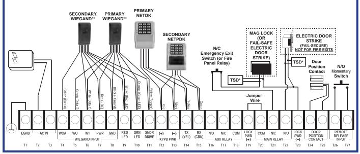
\*TSD = Transient Suppression Device (two supplied): Mount the TSD as close to the device to be protected as possible. \*\*Example device shown: HID ProxPoint<sup>®</sup> Plus Model 6005B.
