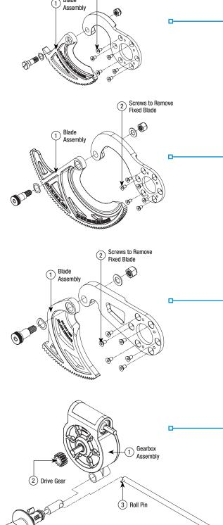
Screws to Remove Fixed Blade
