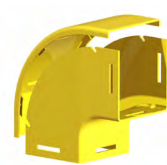
SRS-ELKT-DN90-YL-C SpeedPRO™ Vertical Elbow with cover, 90° down, 50 mm x 50 mm (2 in x 2 in), yellow
