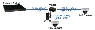
Vi3103 allows for the transmission of two cameras over a single camera run or adding a new camera close to an existing camera.
