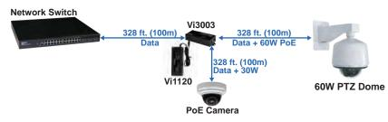
*Vi3003 allows for the transmission of two cameras over a single camera run or adding a new camera close to an existing camera.*
