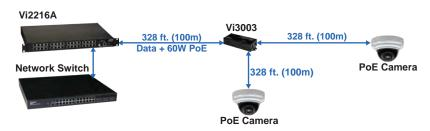
*Vi3003 allows for the transmission of two cameras over a single camera run or adding a new camera close to an existing camera. The PoE Midspan provides power to the Vi3003 and both cameras.*
