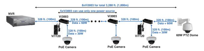
A total of 9 IP addresses can be accessed on a single cable run, eliminating the need for network switches.
