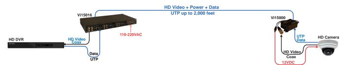
The Vi15000 series can provide HD video, data and power transmission over UTP at istances up to 2,000 feet eliminating the need for camera local power supply.
