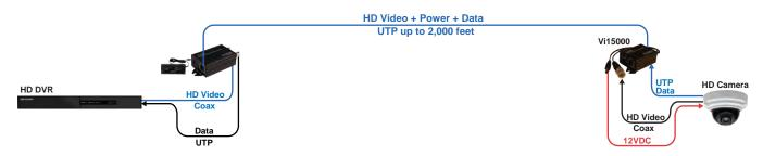
The Vi15000 series can provide HD video, data and power transmission over UTP at istances up to 2,000 feet eliminating the need for camera local power supply.
