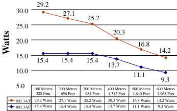
\* Results charted were calculated using four pair 24awg Cat5e cabling and power sourcing equipment using IEEE 802.3AF standard with starting voltage of 48Vdc and IEEE 802.3AT standard with starting voltage of 54Vdc. PoE Switches with internal power and current limits may change individual results.
