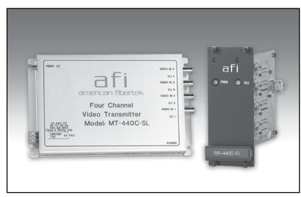
The American Fibertek 440C-SL Series transmit four channels of high-quality, FM video on one singlemode optical fiber at 1300 nm. Designed to be completely transparent to all camera and monitor manufacturers, the system requires no field adjustments at installation or additional maintenance thereafter. Diagnostic indicators provide a quick visual indication of system status.
