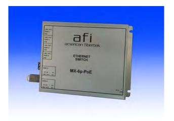
The American Fibertek MX-6p-PoE Series transmits and receives (4) copper 10/100 Base-TX Ethernet signals at the RJ45 ports and (2) optical 1000 Base-X over 1 or 2 optical fibers. The system is comprised of two or more units forming a communications link
