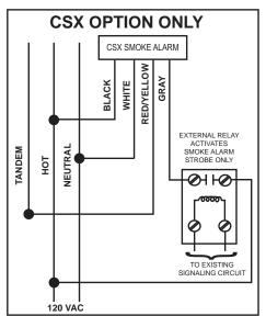
*NOTICE:* Each CSX model strobe to be activated must be connected to the external relay using the GRAY wire.
