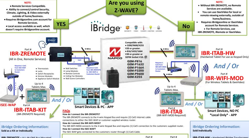
IBR-ZREMOTE - ALL-IN-ONE Bus Mounted module for remote control, Upload/Download of security system, IP Reporting, PLUS control of Z-Wave devices (lights, locks, thermostats, etc.).
