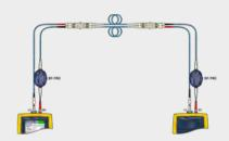
Unlike competitive fiber adapters which measure length and two loss measurements per Autotest, DTX is the only fiber test solution that measures length and four loss measurements per Autotest - all in about 12 seconds.
