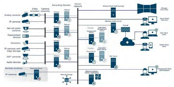
RECORDING SERVER / FAILOVER RECORDING SERVER Powerful, high performing software built on a native 64-bit Windows service supporting minimum 3.1 Gbit/s recording rate.
