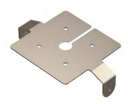
The AccelTex Solutions Cisco AIR-ANT2513P4M-N Adapter Plate for the ATS-APANTARTMNT-UNIV1 allows the Cisco 2513P antenna to mount to the AccelTex AP and Antenna Articulating Mount. The adapter plate ships with the fasteners to attach the Cisco antenna to the adapter plate. The original antenna plate that shipped with the AccelTex Mount is discarded and replaced with this adapter plate.
