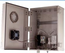
The AccelTex Solutions Heated & Cooled PoE enclosure allows an access point to be installed in an outdoor or other temperature-limiting environment. The heater, fan and AP are all powered by a single PoE cable run from the network switch.
