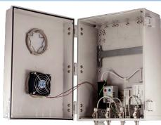
The AccelTex Solutions Heated & Cooled PoE enclosure allows an access point to be installed in an outdoor or other temperature-limiting environment. The heater, fan and AP are all powered by a single PoE cable run from the network switch. The enclosure ships ready for an AP and external antenna installation.
