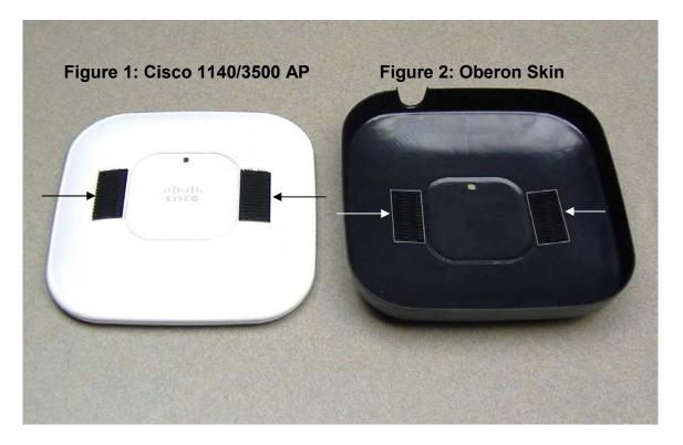
The following procedure should be used to install the Oberon skin on the Cisco 1140/3500 access point.
