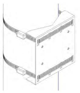
Figure 1 - Pole Mounting Bracket
