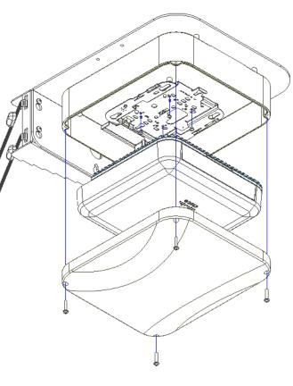
Step 3 – Fasten the enclosure to the Right Angle Bracket
