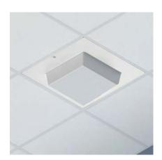
Locking suspended ceiling enclosure secures general purpose telecom/zone equipment and used for attaching (2) directional antennas and APs. Secure active equipment including Optical Network Terminals (ONTs), small workgroup switches, APs, DAS remote access units (RAUs), and directional antennas. The dome is ABS plastic and virtually transparent to wireless signal. Fire-stopped openings for the multi-fiber array modules and multi-copper connector modules used in pre-terminated solutions.
