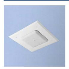
Model 1042-CCOAP3800 provides the simplest way to recess APs into the ceiling for an aesthetic, professional installation. A cutout is made in the ceiling and the back-box is fastened to the ceiling (remodel). The AP fastens to the AP-specific trim, and the trim to the back-box. The AP is recessed into the ceiling much like a recessed light fixture. AP trim can be easily swapped for new trim if the AP brand or model changes in the future. See specs for AP-specific model names.
