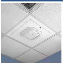
This locking retrofit door is designed to provide a convenient way to mount and secure wireless access points in 1047 Series AP enclosures. To remove the old door, simply unlock the door, open the door to a 90° angle, align the tabs of the door mount to the slots in the back-box hinge opening, and slide the door forward. Simplify equipment replacement without lifting ceiling tiles.
