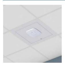
Locking, 2' x 2' suspended ceiling tile enclosure mounts and secures wireless access point and DAS remote units with non-detachable or internal antennas. This steel enclosure replaces a standard ceiling tile, and its larger back-box is suitable for larger access points and antennas. The interchangeable door simplifies access point and antenna changes. Access points can be mounted in the door or inside the enclosure with the configurations with the dome.
