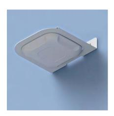
Many AP manufacturers recommend APs be mounted in a horizontal orientation. Secure APs from most manufacturers in areas where wall mounting may be required, such as residence halls, hotels, and other hard lid venues. The AP is partially recessed into the right-angle bracket, exposing only the antenna face of the AP. Conduit, raceways, and cable can be terminated in the bracket. The AP can be locked in place using the manufacturer's locking features. Specify AP and model when ordering.
