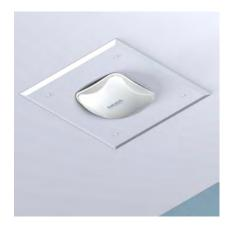
Model 1043 offers the simplest way to recess APs into the ceiling for an aesthetic, professional installation. A cutout is made in the ceiling and the backbox is fastened to the ceiling joists (new construction). The AP fastens to a AP-specific trim, and the trim to the back-box. The AP is recessed into the ceiling much like a recessed light fixture. Access point trim can be swapped easily for new trim if the AP brand or model changes in the future. See specs for AP-specific model names.
