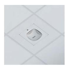
Locking 2' x 2' suspended ceiling enclosure secures APs with integrated antennas. Replaces a standard ceiling tile and is UL listed for installation in the plenum space. Interchangeable doors mount leading vendors' APs nearly flush to the ceiling for a professional, aesthetic installation. Interchangeable doors simplify moves, adds, and changes without lifting ceiling tiles. The -T features a flange beveled at the edge to mimic a tegular ceiling tile used in recessed grid suspended ceilings.
