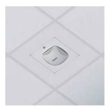
Economical, locking 2' x 2' suspended ceiling tile enclosure mounts and secures APs flush to the ceiling. The interchangeable door simplifies access point and antenna moves, adds, and changes without lifting ceiling tiles. Access points can be mounted in the door or inside the enclosure with the configurations with the ABS dome. "-T" version matches tegular ceiling tiles used in recessed grids. Specify -T version for professional, aesthetic installation in recessed grid ceilings.
