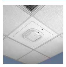
Locking, 2' x 2' suspended ceiling tile enclosure mounts and secures wireless access point and DAS remote units with non-detachable or internal antennas. This steel enclosure replaces a standard ceiling tile, and its larger back-box is suitable for larger access points and antennas. The interchangeable door simplifies access point and antenna changes. Access points can be mounted in the door or inside the enclosure with the configurations with the dome.
