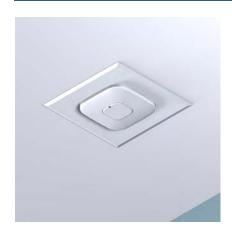
Model 1042-CCOAP provides the simplest way to recess APs into the ceiling for an aesthetic, professional installation. A cutout is made in the ceiling and the back-box is fastened to the ceiling (remodel). The AP fastens to the AP-specific trim, and the trim to the back-box. The AP is recessed into the ceiling much like a recessed light fixture. AP trim can be easily swapped for new trim if the AP brand or model changes in the future. See specs for AP-specific model names.
