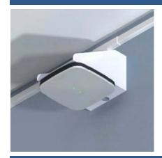
This right-angle mounting bracket has sidewalls to help conceal cabling and can be placed directly over data outlet. Quickly install AP in preferred horizontal orientation. Mounting features for Cisco and Aruba Networks APs, with universal T-bar for most other vendors' APs. White powder-coated steel. Ideal for hard lid environments such as residence halls.
