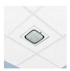
Locking, 2' x 2' suspended ceiling tile enclosure mounts and secures wireless access points flush to the ceiling. The interchangeable door simplifies access point and antenna moves, adds, and changes without lifting ceiling tiles. Access points can be mounted in the door or inside the enclosure with the configurations with the ABS dome. "-T" version matches tegular ceiling tiles used in recessed grids. Specify –T version for professional, aesthetic installation in recessed grid ceilings.
