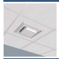
Locking multimedia ceiling enclosure mounts and secures digital media gateways, APs and other components in the ceiling. Once installed, this ceiling enclosure permits controlled access to components without lifting ceiling tiles. Interchangeable retrofit doors permit easy vendor and technology migrations. Steel enclosure fits into a cutout in the ceiling tile.
