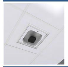
Locking multimedia ceiling enclosure mounts and secures digital media gateways, APs and other components in the ceiling. Once installed, this ceiling enclosure permits controlled access to components without lifting ceiling tiles. Interchangeable retrofit doors permit easy vendor and technology migrations. Steel enclosure fits into a cutout in the ceiling tile.
