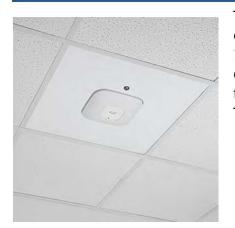
This locking, suspended ceiling tile-like mount is designed to provide a convenient way to secure Cisco wireless access points in the ceiling. Many of the 106X series AP mounts feature a unique, patented locking mechanism which draws the AP part way into the mount, exposing only the antenna face of the AP, for the ultimate in wireless coverage, aesthetics, and physical security. Textured, white powder-coated steel and aluminum construction.
